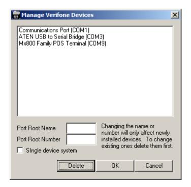
This shows all the communication ports on the machine, whether the devices are connected or not.
